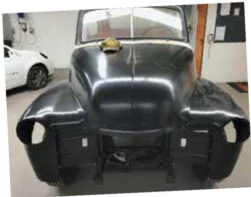
Due to a lack of fit accuracy, the new parts from the USA caused a lot of work.
